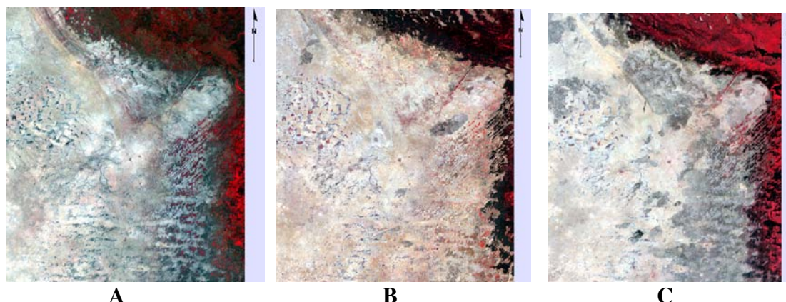
Figure 2: 30m pixel 1984 Landsat5 TM 234 band composite of the study area A), 30m pixel 1992 Landsat4 TM 234 band composite of the study area B), and 15m pixel 2000 Landsat5 TM 234 band composite of the study area C).
