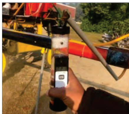
Fig. 5. Discharge rate measurement and spray tip pressure tester
