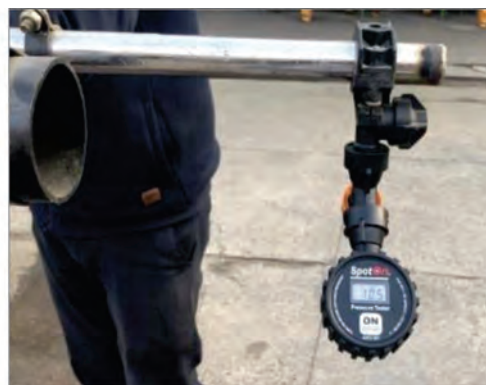
Fig. 5. Discharge rate measurement and spray tip pressure tester
