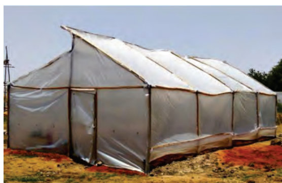
Fig. 3. Developed bamboo polyhouse for Telangana semi-arid tropics (Source: Gopi et al. , 2019)
