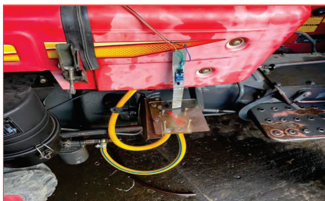
Fig. 2. Fuel consumption meter mounted with plastic slit covered with reflector tape
