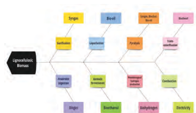
Fig. 4. Conversion pathways for LCBs into bioethanol, biogas, biohydrogen, bio-oil, electricity
