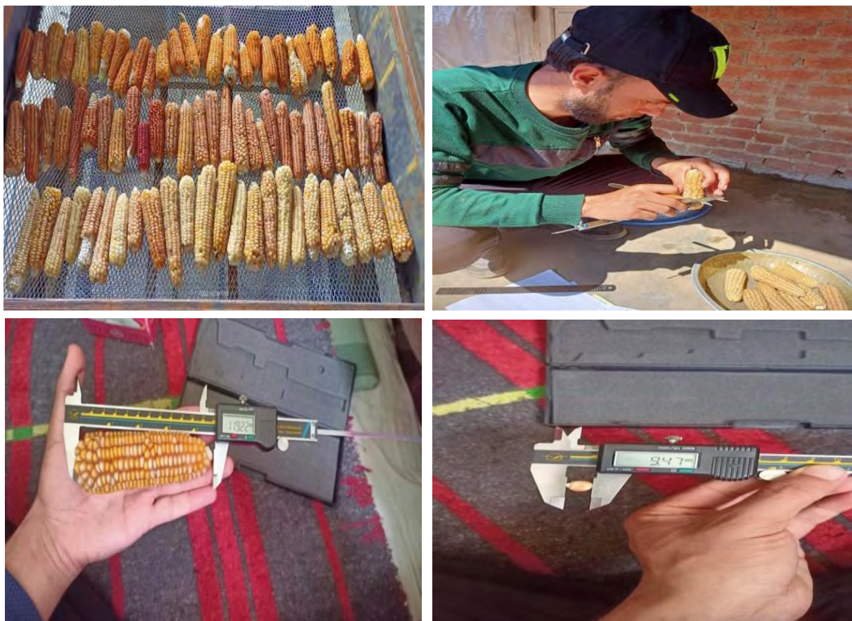
Fig. 2: Measurement of tri-axial dimensions of maize varieties with digital Vernier Calliper
