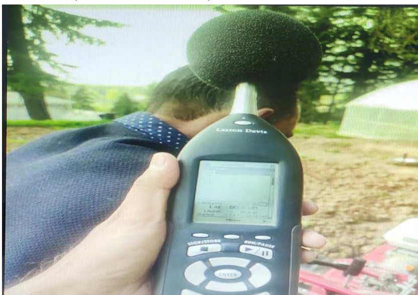
Fig.1: Measurement of sound pressure level at operator's ear level during weeding operation
