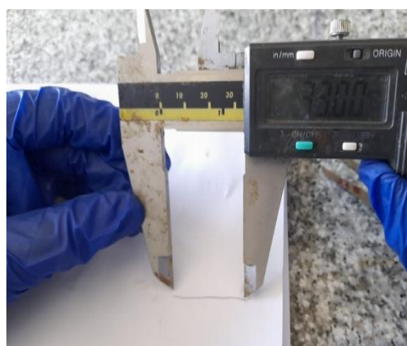
Fig. 3: Measurement of thread using vernier calliper for Rainbow Trout and Mirror Carp
