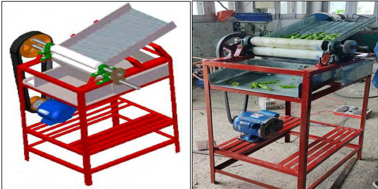
Fig. 2: 3-D view of pea depodding machine
