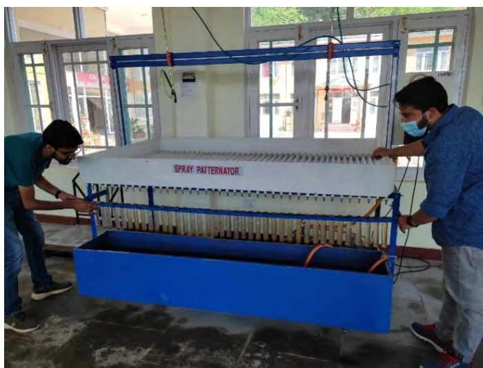
Fig 3: Determination of discharge, swath width and spray pattern using Spray patternator
