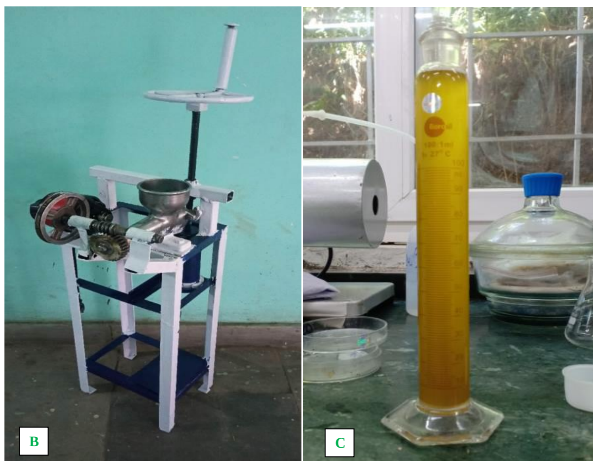
Fig. (B) Developed prototype of walnut kernel oil extractor and (C) walnut oil sample extracted
