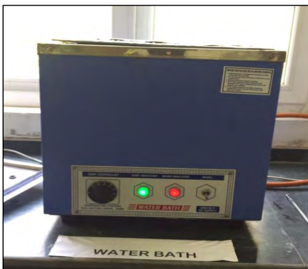
Fig.2: Water bath used as refractance window dryer
