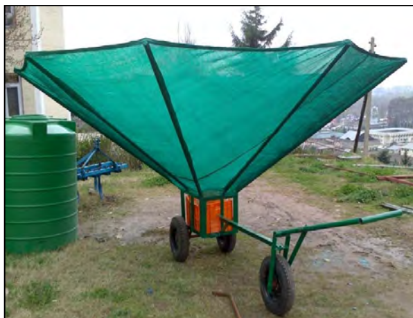
Fig. 2: A view of the developed apricot catch net (inverted Umbrella)
