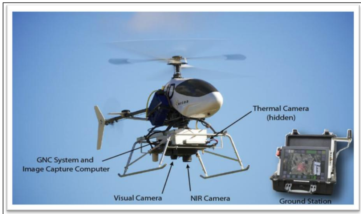
Fig. 4: Phenocopter-A pilotless aircraft for remote sensing
